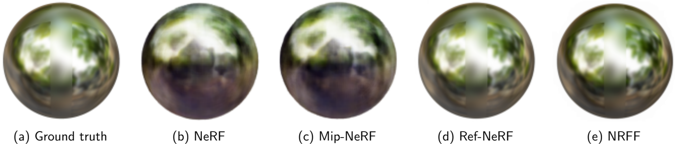
Figure 1: Foundational models NeRF and Mip-NeRF fail to render highly specular surfaces accurately, also unable to represent different specular roughness of the stripes around. Ref-NeRF and NRFF are able to render substantially more accurate details based on physical modeling of the reflection phenomena.
