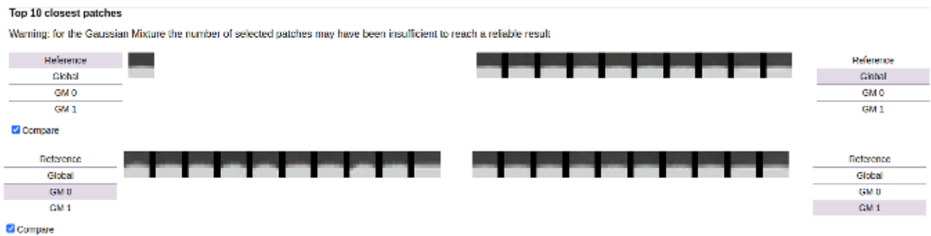
Figure 5: Above: seed patch and its top ten closest patches. Below, the 10 patches with highest probability of each component of the Gaussian mixture.
