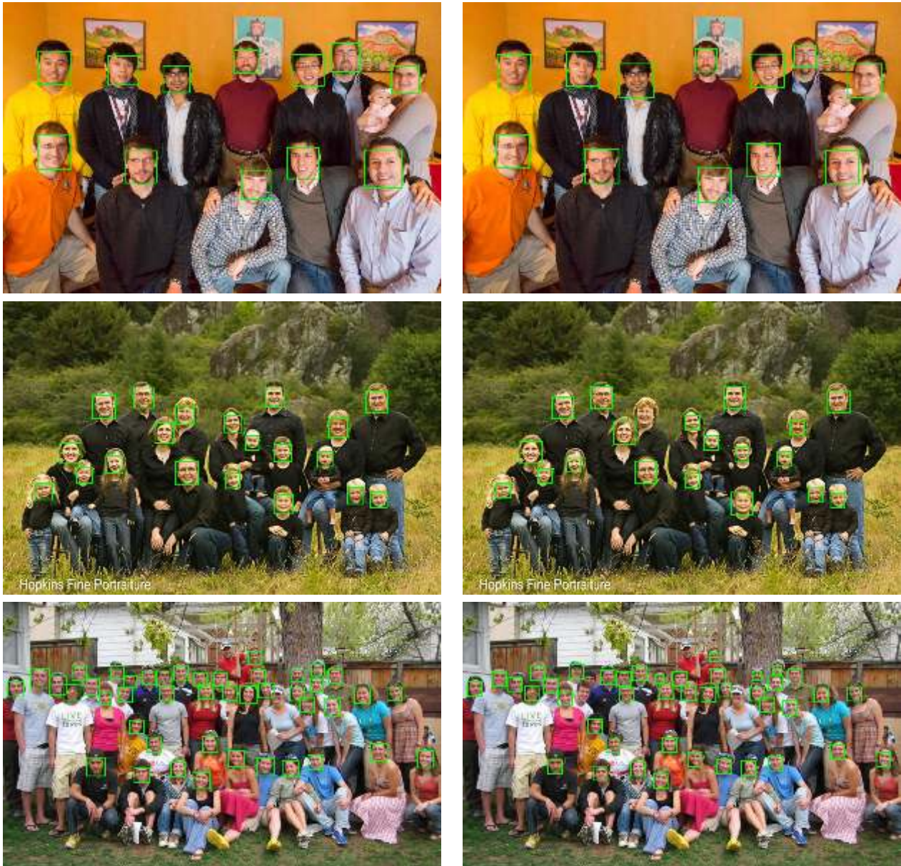
Figure 10: Results with frontal faces. Left, results of the proposed method for NFP_{\max} = 1 . Right, result of a full-cascade of classifiers without adaptive detection thresholds [19].
