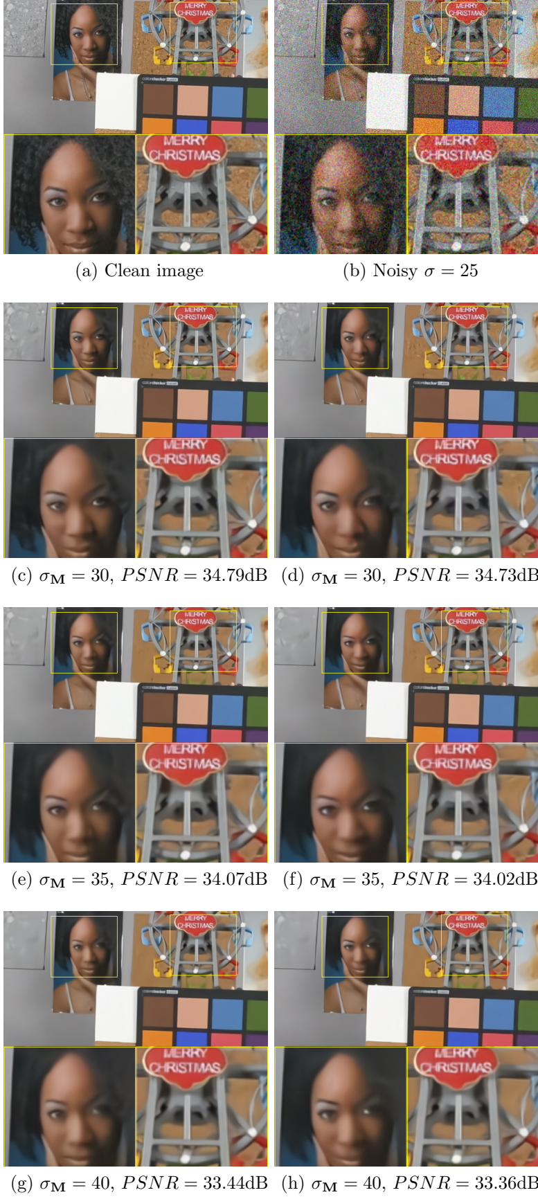
Figure 9: Comparison of models with and without orthogonalization in case of noise mismatch. Left: regularized model. Right: model with no regularization. The noise level \sigma_M indicated in the noise map mismatches the actual noise in the input \sigma . The regularized model performs marginally better than the one without regularization as it recovers slightly more details and structures.
