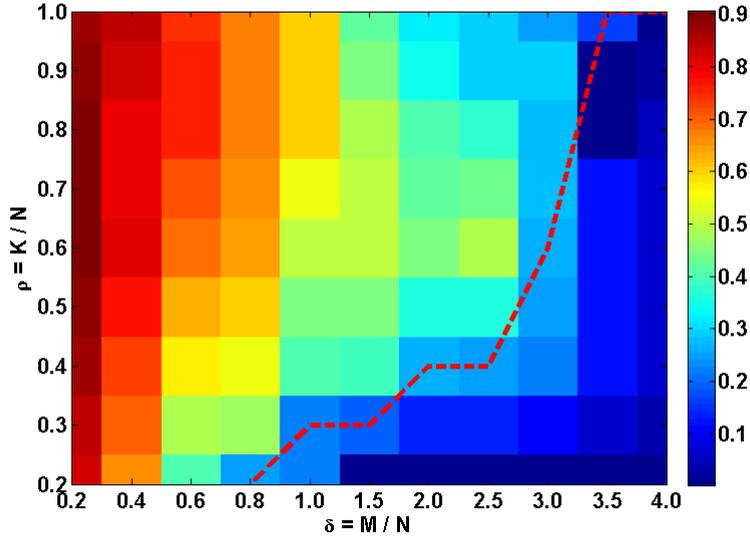
Figure 2: prSAMP phase transition plot for solving the phase retrieval problem using a binary measurement matrix. Here,  $N = 256$  and SNR of 30 dB are considered in all the experiments. The performance criterion is NMSE which is selected out of 50 independent trials. The red dashed line represents a transition from failure to success by applying a threshold of 0.2.
