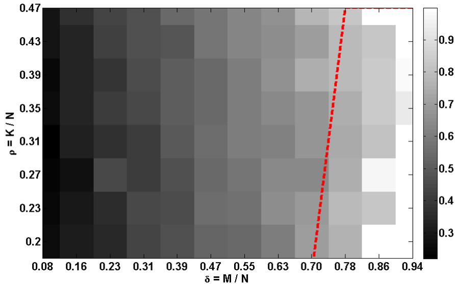
Figure 5: prSAMP phase transition plot for solving the phase retrieval problem, with a binary input, using a complex measurement matrix. Here,  $N = 256$  and SNR of 30 dB are considered in all the experiments. The performance criterion is the correlation, which is selected as the best out of 50 independent trials. The red dashed line represents a transition from failure to success by applying a threshold of 0.8.
