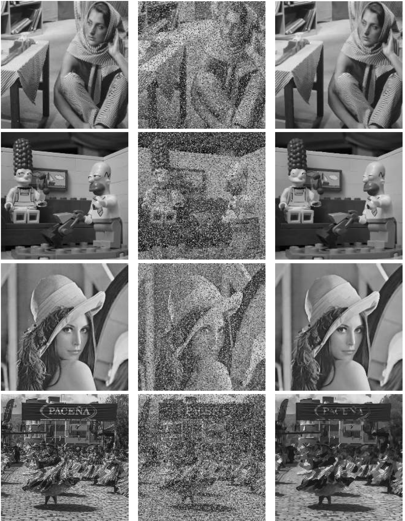
Figure 7: Restored images for an intensity of impulse noise p = 40\% . For each column, from left to right: original image, noisy image, our method.
