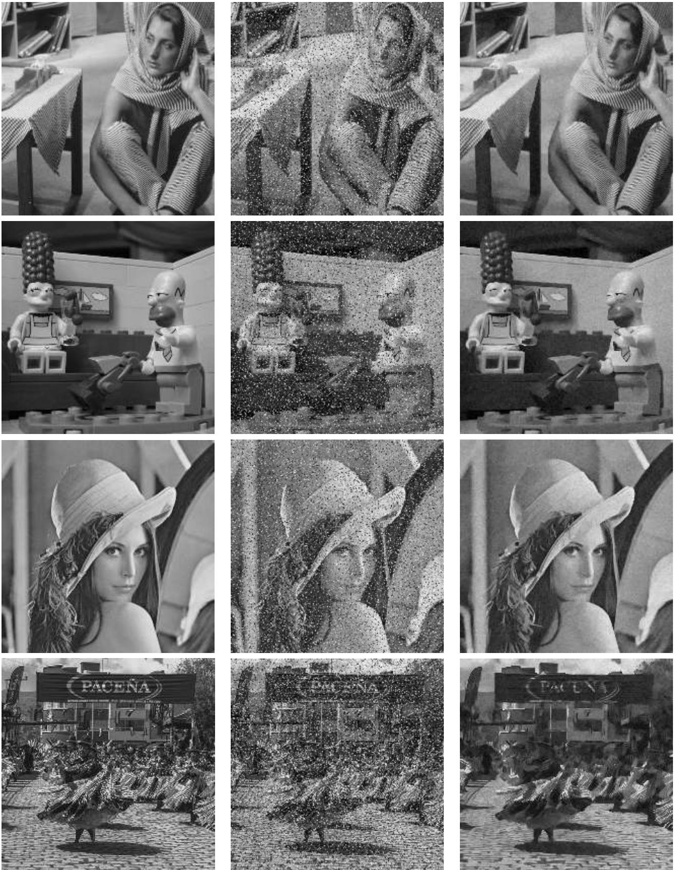
Figure 12: Restored images for a Gaussian noise of standard deviation \sigma = 20 and an intensity of impulse noise p = 20\% . For each column, from left to right: original image, noisy image, our method.
