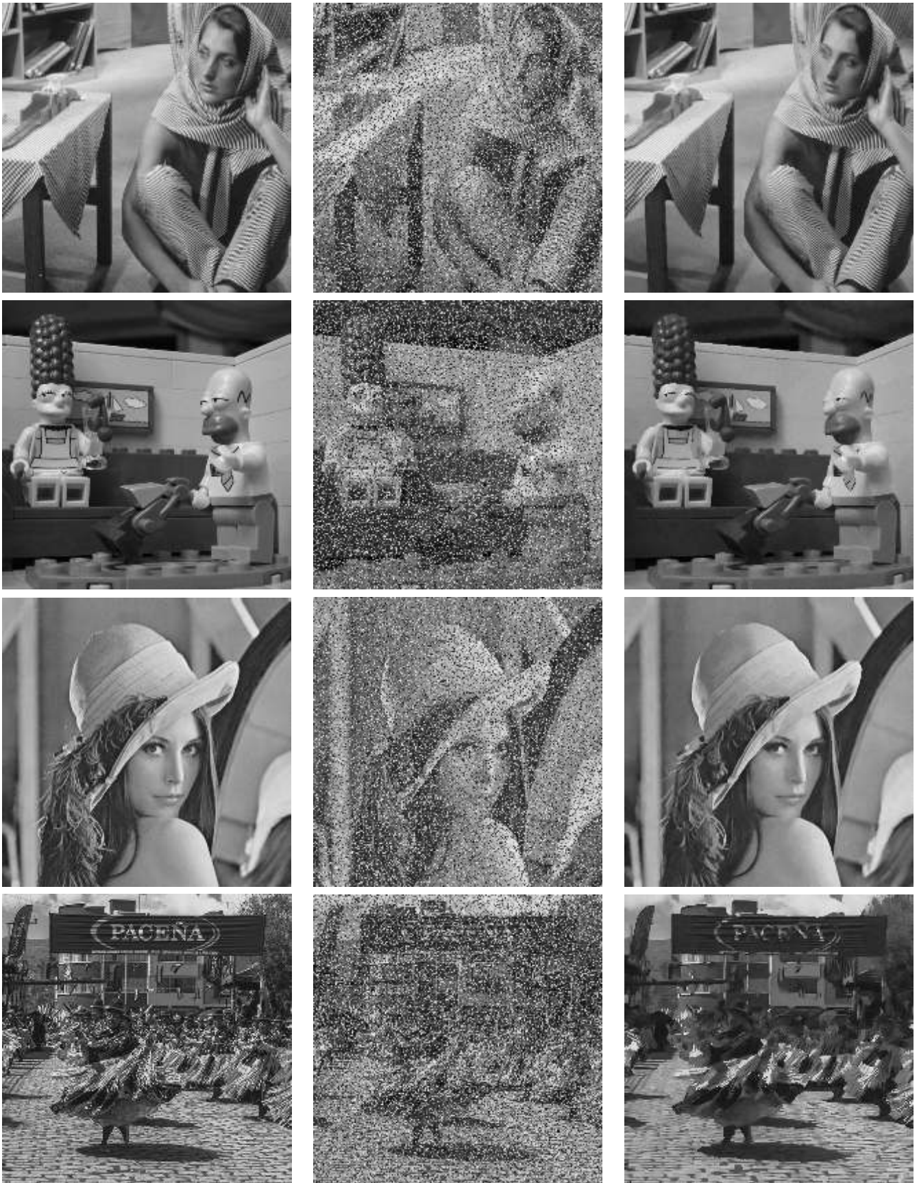
Figure 10: Restored images for a Gaussian noise of standard deviation \sigma = 10 and an intensity of impulse noise p = 40\% . For each column, from left to right: original image, noisy image, our method.
