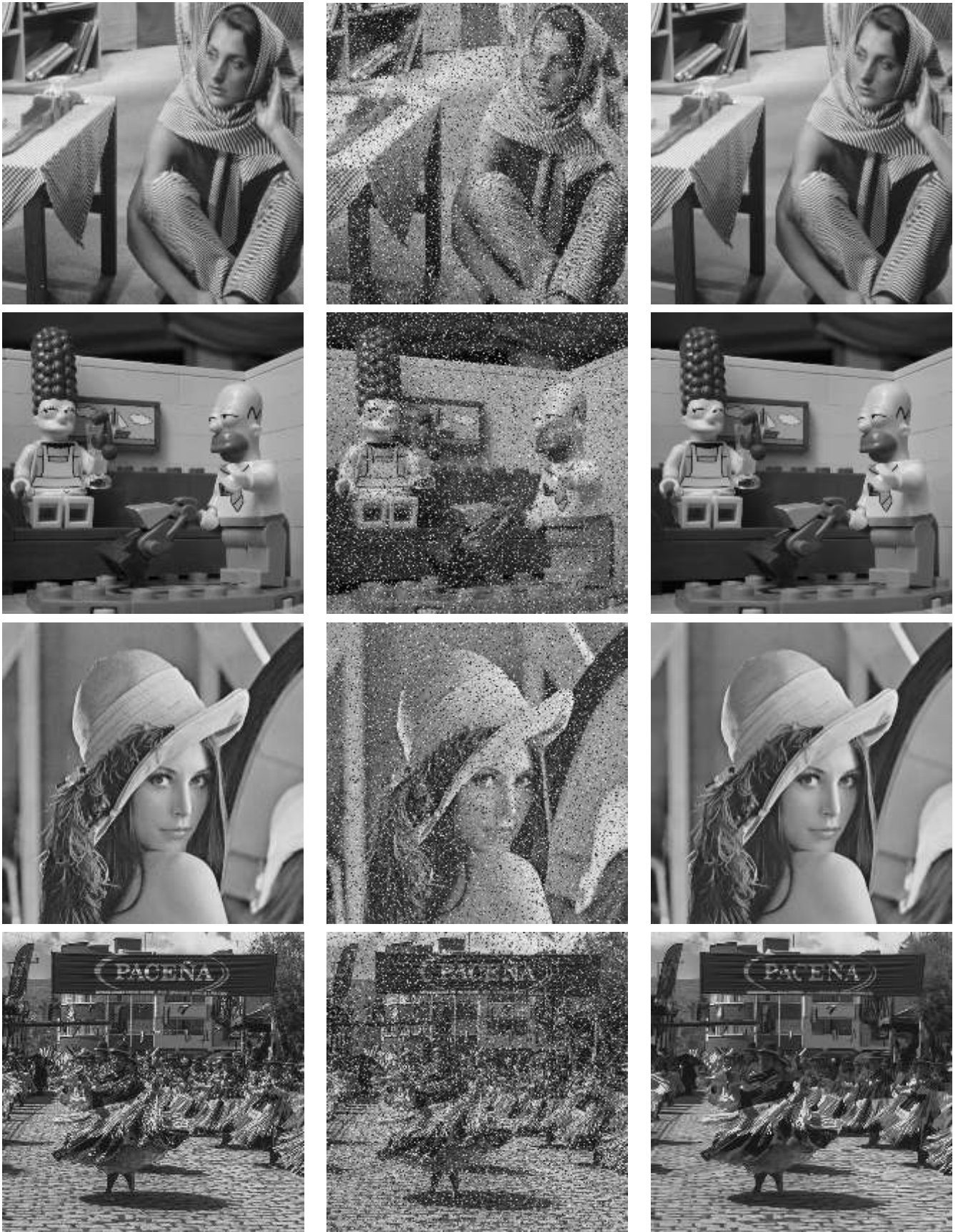
Figure 6: Restored images for an intensity of impulse noise p = 20\% . For each column, from left to right: original image, noisy image, our method.
