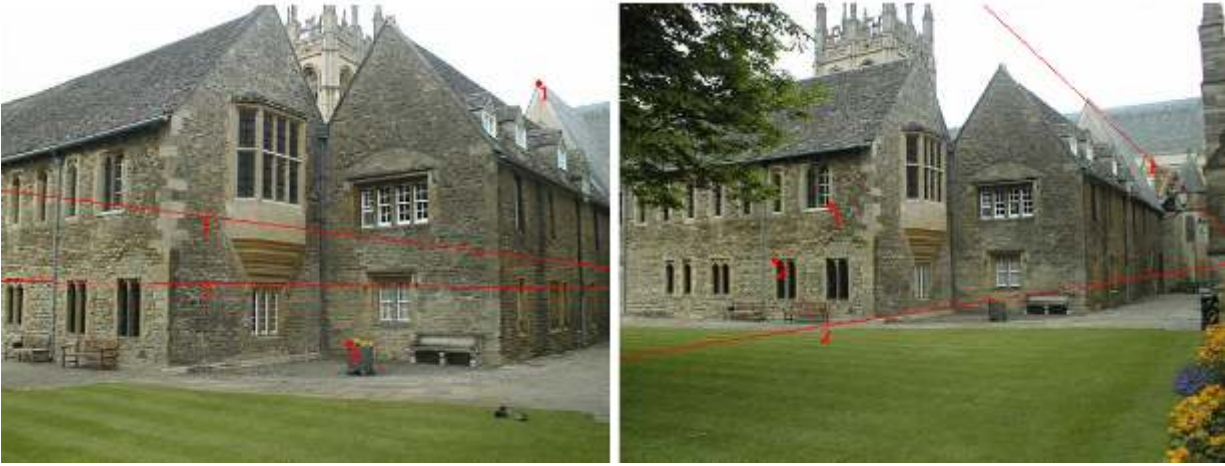
Figure 6: Stereo pair with interactive display of epipolar lines. Line numbers are associated to the same point numbers in the other image (these numbers do not appear in the online demo).
