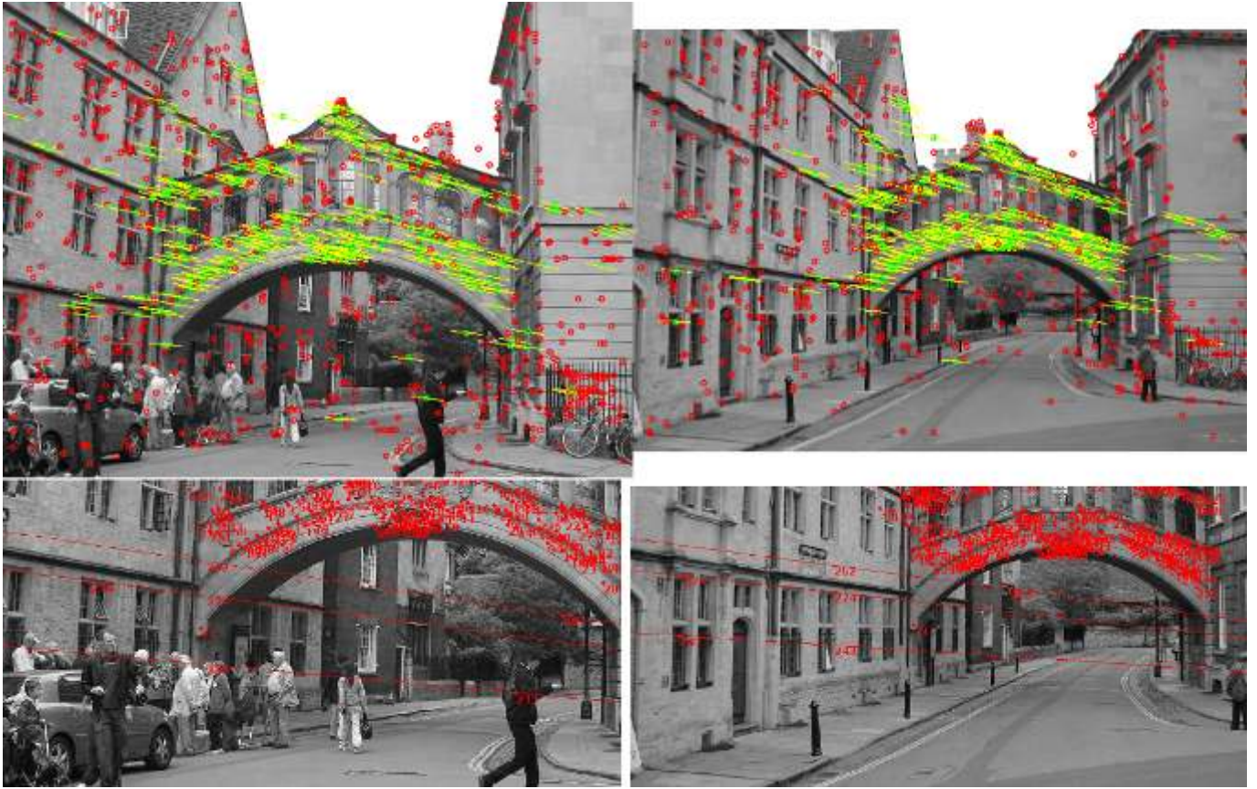
Figure 7: Example of wrong matches still considered as inliers because the epipolar constraint is not very discriminative (pair and correspondences from USAC [16], fundmatrix/test3 ). The top images show all inliers and outliers according to the algorithm. The bottom images show 3 wrong correspondences (243, 262 and 274) that still satisfy the epipolar constraint, and are thus wrongly classified as inliers.
