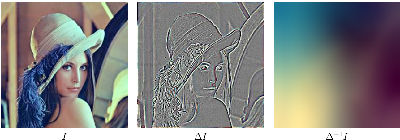
Figure 8: The Laplacian and anti-Laplacian of the same image. Notice that the anti-Laplacian is a very smooth image. The ranges of these three images are respectively [0, 255] , [-5, 5] and [-127, 127] . For display purposes, these ranges have been re-scaled to fill the interval [0, 255] .
