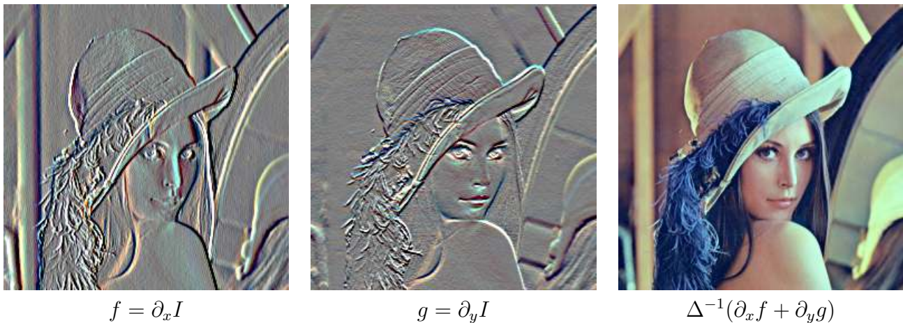
Figure 9: The Poisson editing method allows to recover an image (up to an additive constant), from its gradient.
