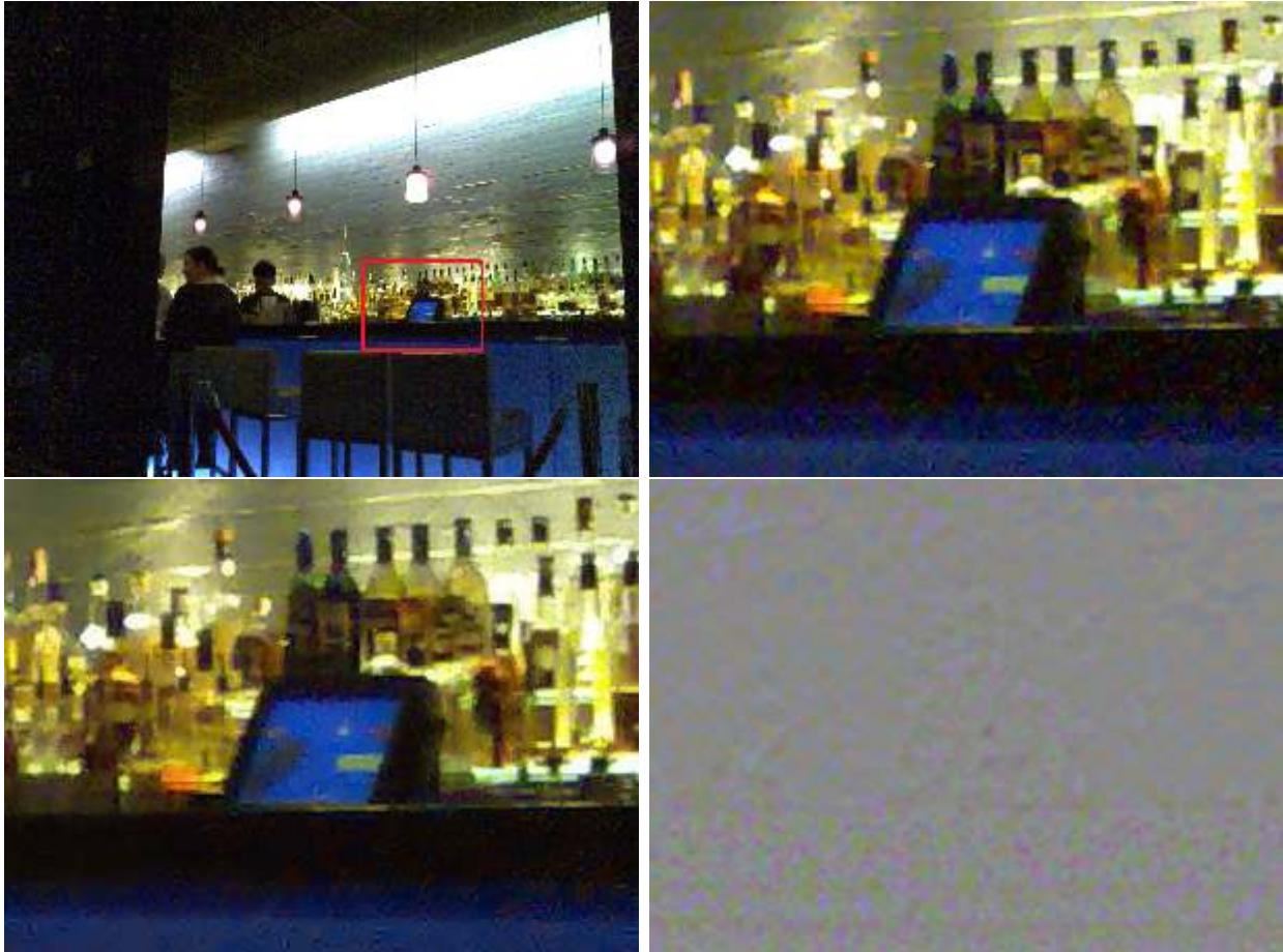
Figure 21: Blind denoising on “Bar”, using three scales. From left to right, top to bottom : input noisy image, crop of the noisy image, crop of the output denoised image, crop of the difference image.
