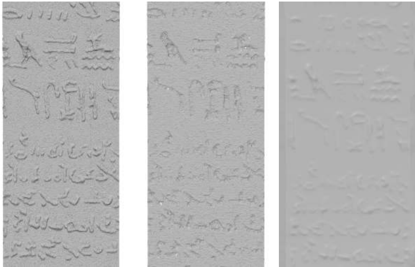
Figure 5: Comparison of the Scale-Space Meshing (left) with the standard Ball Pivoting Algorithm (middle) and Poisson Reconstruction (right)
