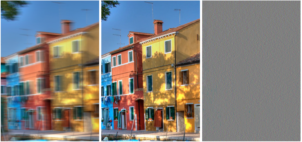
Figure 13: Motion-invariant photography code. Left: observed image. The blur interval length is equal to 52 pixels here. Center: reconstructed image (RMSE = 2.11). Right: residual noise (difference between ground truth and reconstructed, dynamic normalized on [0, 255] by an affine contrast change).
