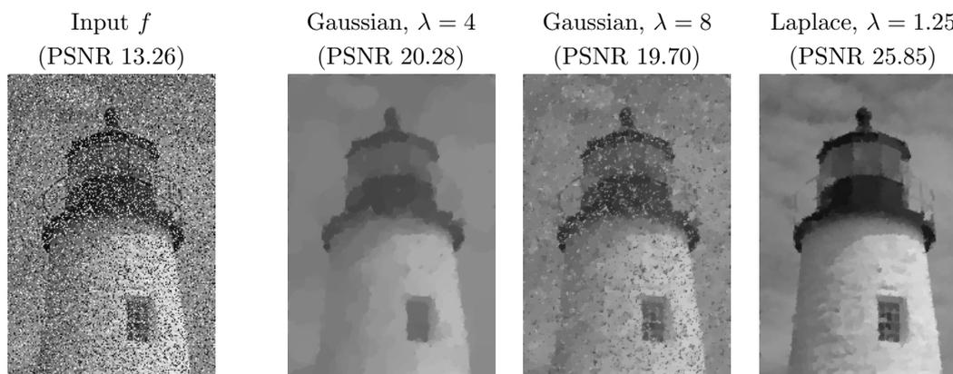
The Laplace model is more effective for removing impulsive noise.
