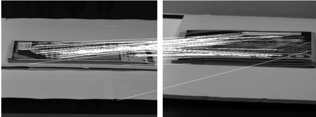
90 correct matches, 4 outliers. The matches were obtained by the *Affine SIFT* method (ASIFT), a variant of the SIFT method.
