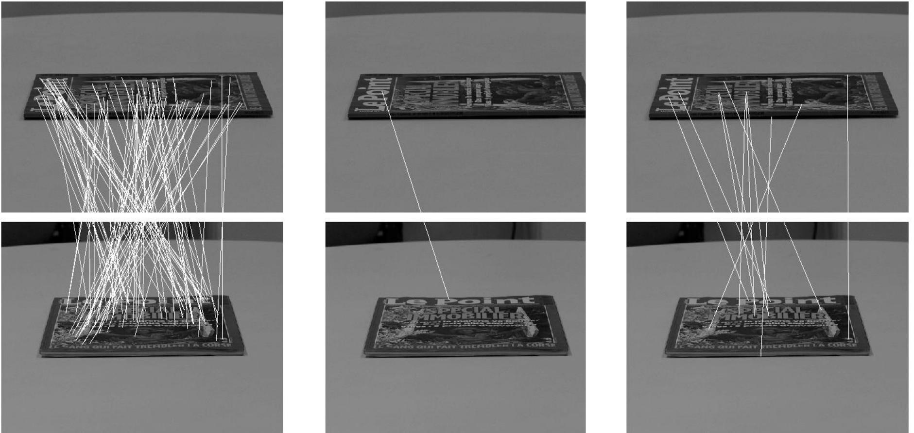
Correspondences between the magazine images taken with absolute tilts  $t_1 = t_2 = 4$  with longitude angles  $\phi_1 = 0^\circ$  and  $\phi_2 = 90^\circ$ , transition tilt  $\tau = 16$ . Number of correct matches: ASIFT (left)—88; SIFT (middle)—1; MSER (right)—9.
