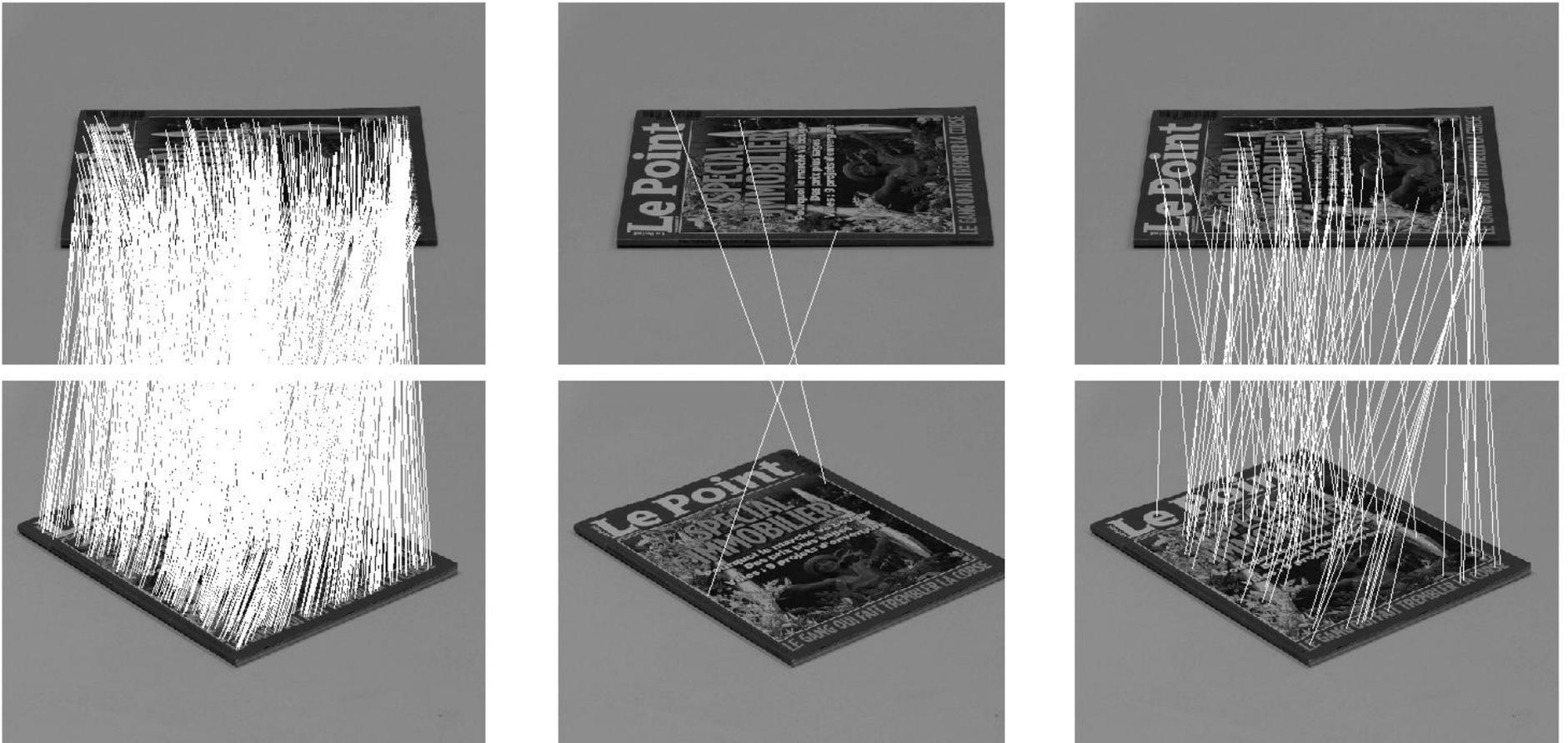
Correspondences between the magazine images taken with absolute tilts  $t_1 = t_2 = 2$  with longitude angles  $\phi_1 = 0^\circ$  and  $\phi_2 = 50^\circ$ , transition tilt  $\tau = 3$ . Number of correct matches: ASIFT (left)—881; SIFT (middle)—2; MSER (right)—87.
