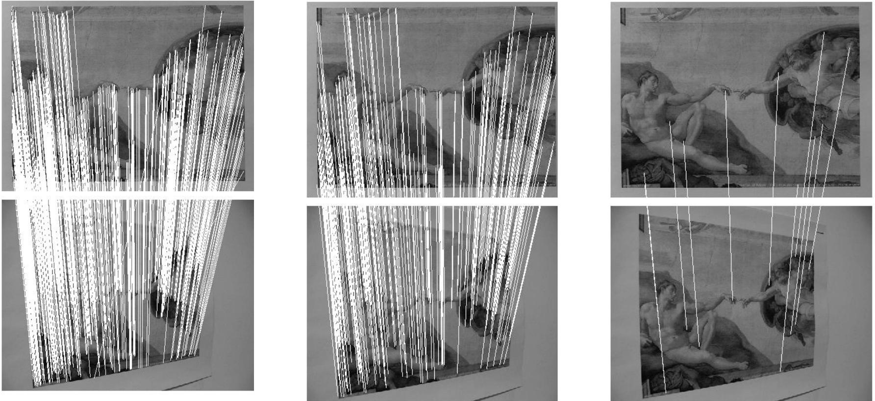
Frontal v.s.  $-45^\circ$  angle, zoom  $\times 1$ : absolute tilt  $t = 2$  (middle),  $t < 2$  (left part),  $t > 2$  (right part). Number of correct matches: ASIFT (left)—624; SIFT (middle)—236; MSER (right)—11.
