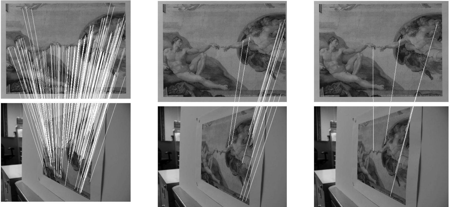
Frontal v.s.  $75^\circ$  angle, zoom  $\times 1$ : absolute tilt  $t = 4$  (middle),  $t < 4$  (left part),  $t > 4$  (right part). Number of correct matches: ASIFT (left)—202; SIFT (middle)—15; MSER (right)—5.
