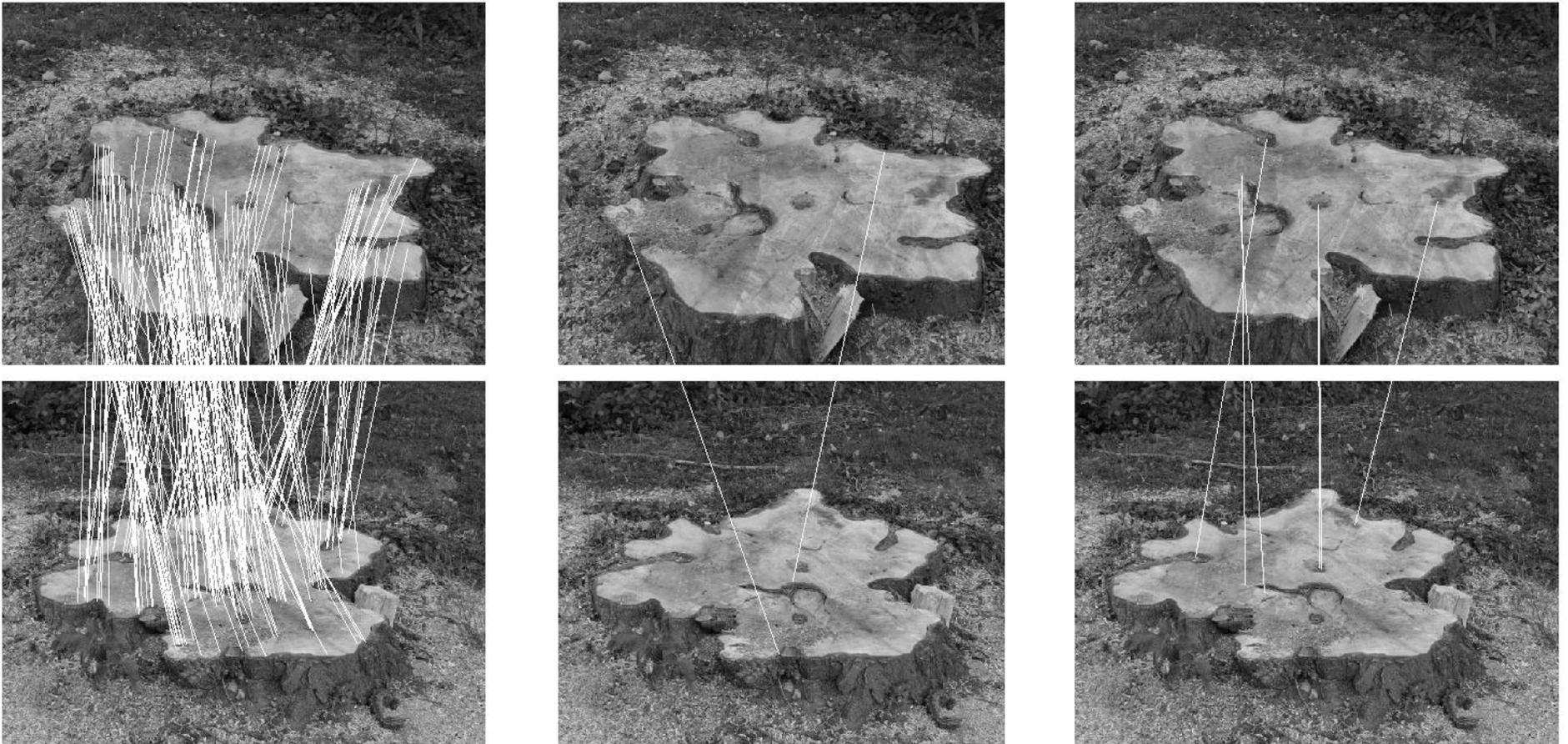
Stump. Transition tilt  $\tau = 2.6$ . Number of correct matches: ASIFT (left)—168; SIFT (middle)—1; MSER (right)—6.
