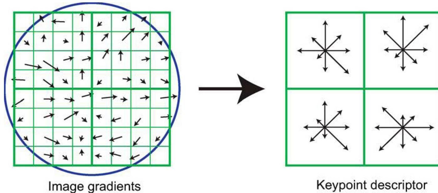
Each key-point is associated a *square image patch whose size is proportional to the scale and whose side direction is given by the assigned direction*. Example of a  $2 \times 2$  descriptor array of orientation histograms (right) computed from an  $8 \times 8$  set of samples (left). The orientation histograms are quantized into 8 directions and the length of each arrow corresponds to the magnitude of the histogram entry.
