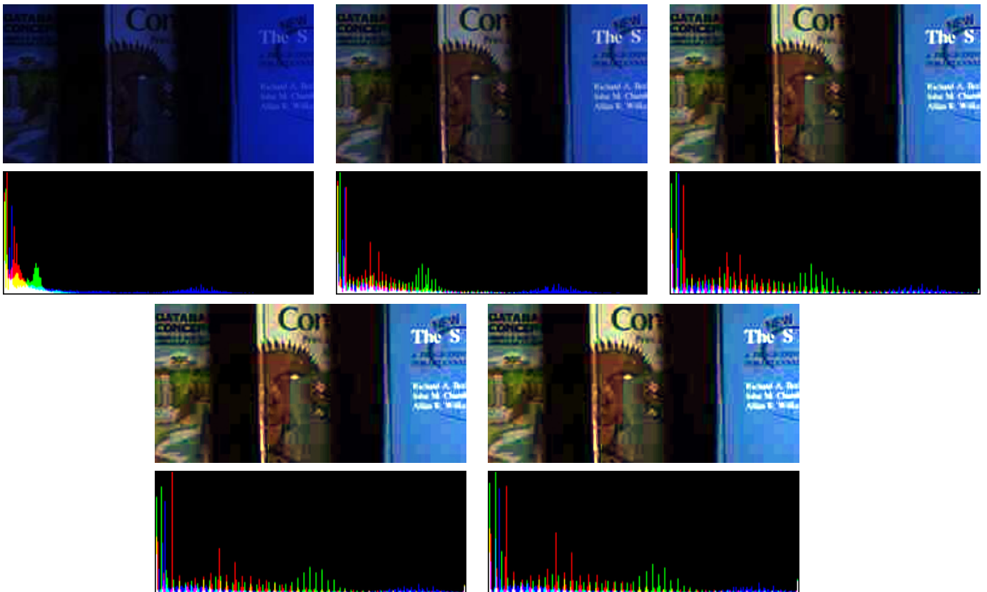
Figure 9: Top row, from left to right: original image, results of the algorithm with s = 0\% and s = 1\% . Third row, results of the algorithm with s = 2\% and s = 3\% . Below each image its RGB histogram is displayed. This image, as the ones in the previous figures, has been used in recent papers on color perception theory (Retinex).
