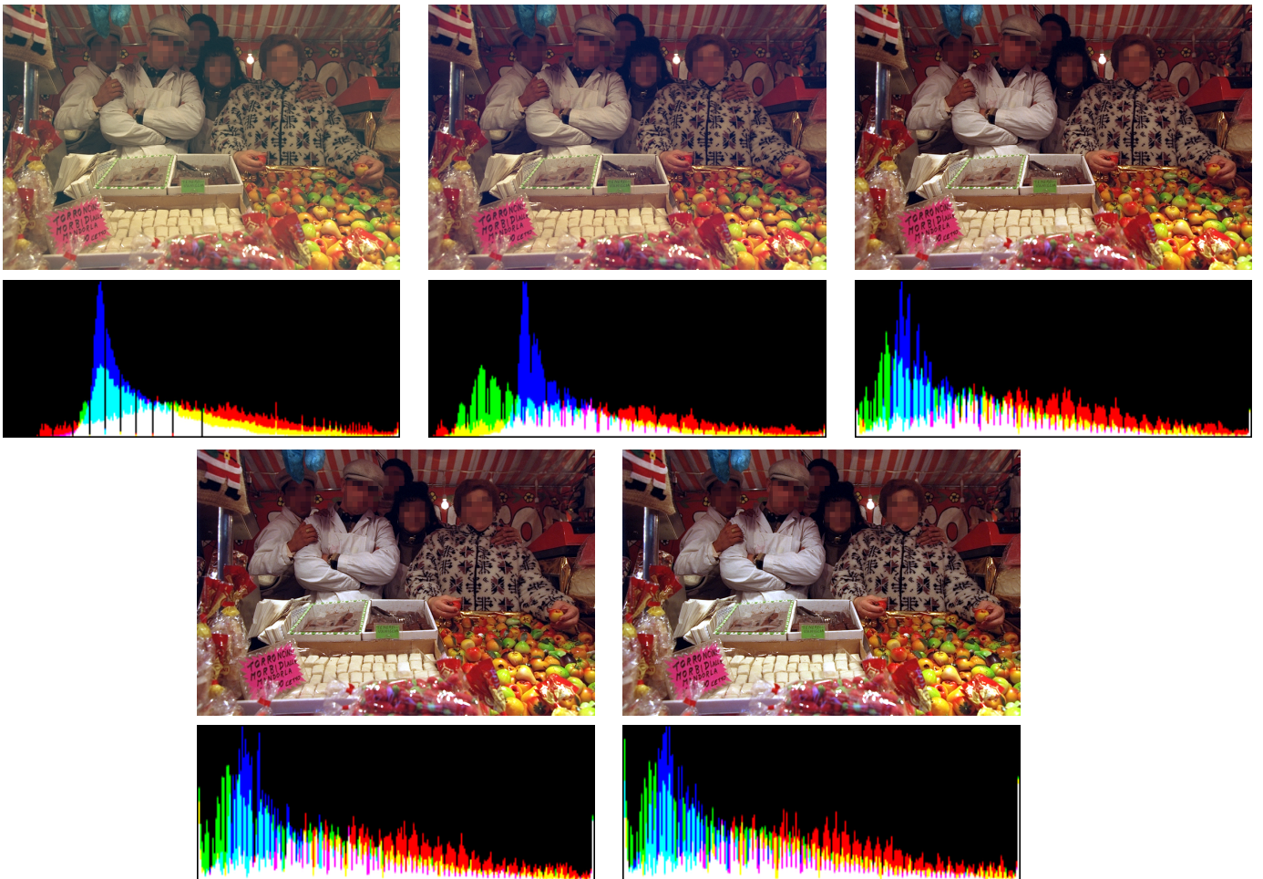
Figure 8: Top row, from left to right: original image, results of the algorithm with s = 0\% and s = 1\% . Third row, results of the algorithm with s = 2\% and s = 3\% . Below each image its RGB histogram is displayed. This image, as the one in the previous figure, has been used in recent papers on color perception theory (Retinex).
